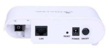
**Extralink 1GE ONU GPON VENUS** is a CPE device functioning in GPON technology. It has one PON and one Gigabit Ethernet port.
